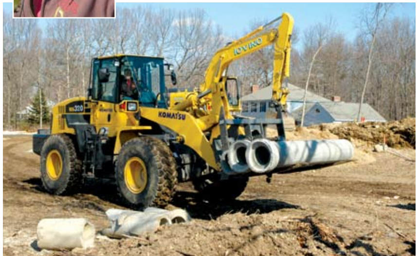
Operator Bob Gettman stacks drainage pipe with a Komatsu WA320-5 wheel loader at a Burlington, Mass., jobsite.
