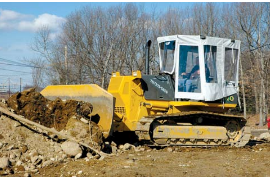
Operator Bob Gettman uses a D41E-6 dozer to stockpile material for future use.
