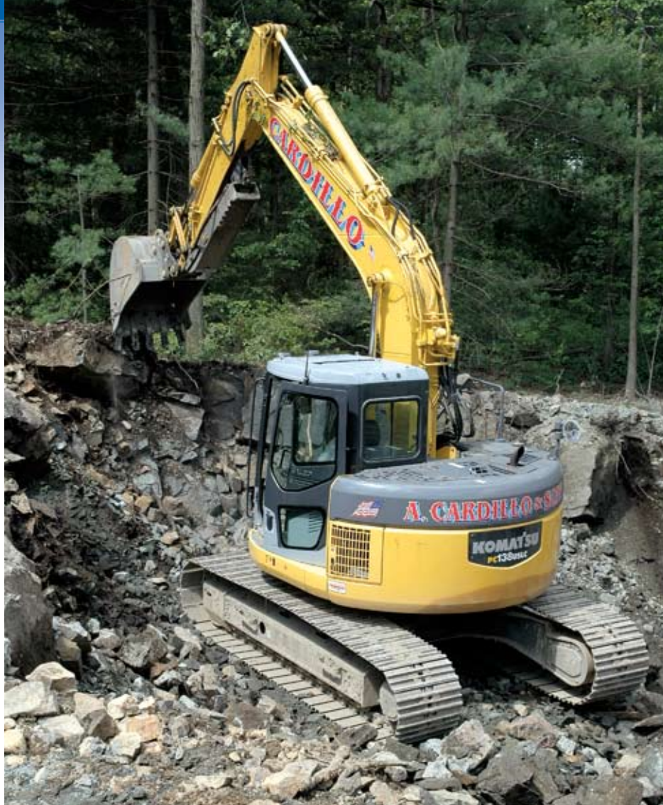
Joe Cardillo uses a Komatsu PC138USLC-3 tight-tail-swing excavator to remove blasted ledge from a homesite. A. Cardillo & Son owns two PC138s, which crews use in limited-space areas. "We're working in tight spots, digging holes and loading trucks, and it's working great," Tony Cardillo said of the excavator.
