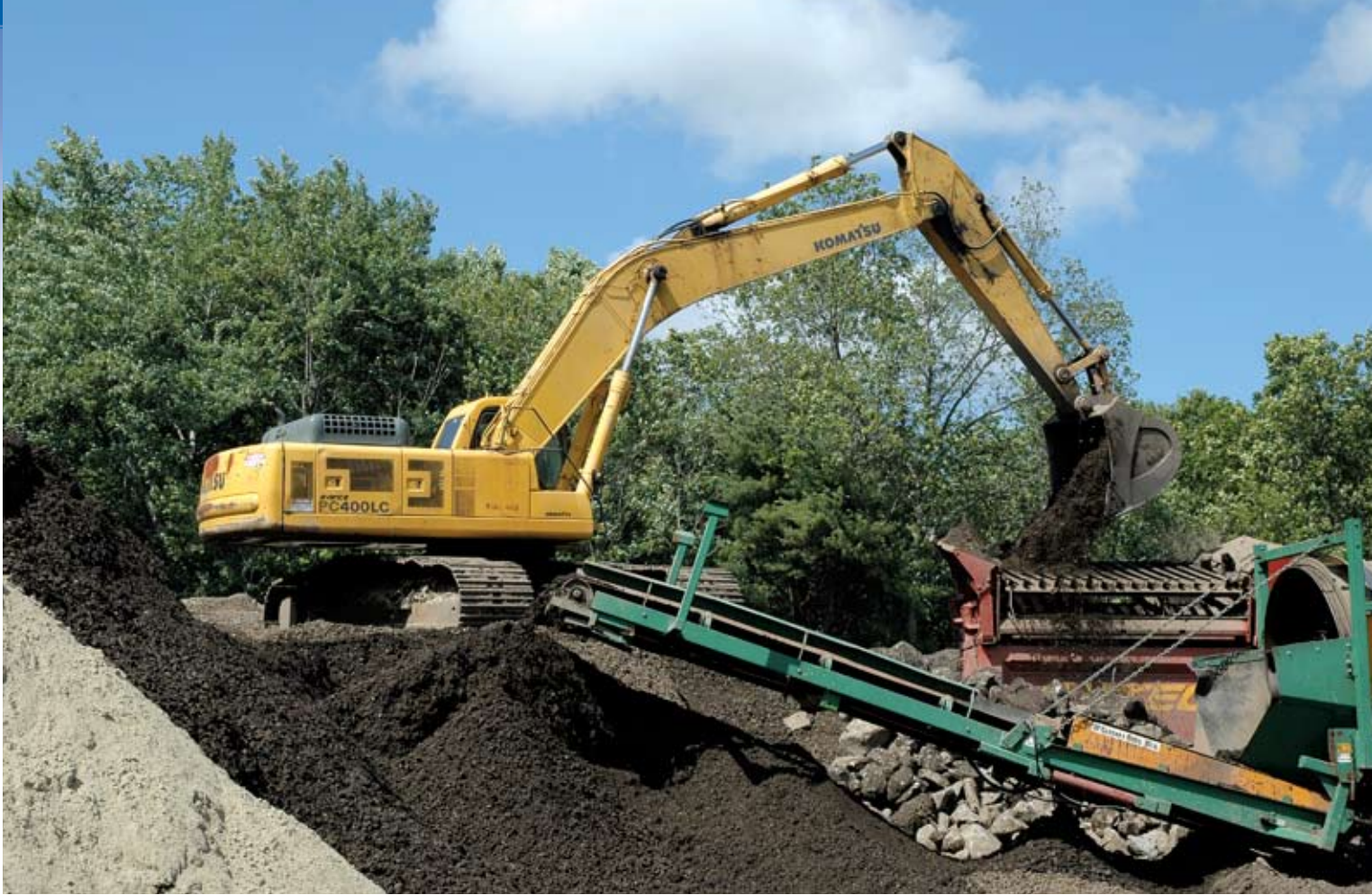
An operator uses Funari Trucking's Komatsu PC400LC-6 excavator to feed loam into the screening plant to produce high-quality screened loam, the company's biggest-selling product. "The excavator has almost 6,000 hours and it's very reliable," said Owner Chris Funari.
