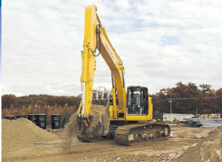
Corliss Construction uses several Komatsu excavators, including this rented 71,647-pound PC308USLC-3. "The zero tail swing allows us to work in tight places," said Project Manager Maan Sinno. "It has great power."
