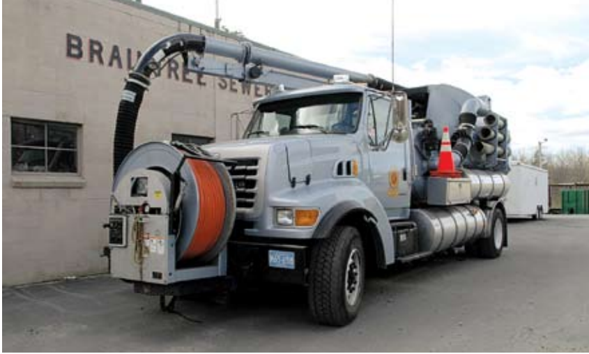
The Braintree Highway and Water & Sewer departments use a Vactor 2100 to flush out sewer mains and vacuum debris from the sewer system.
