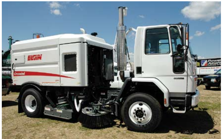
The Elgin Crosswind sweeper on display at the Annual Equipment Show is a four-wheel, dual-engine, truck-mounted, regenerative air sweeper.
