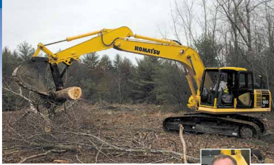
Operator John Briggs uses the Komatsu PC160LC-7 excavator with a thumb attachment to clear trees as part of a project capping one of the town of Exeter's landfills.
