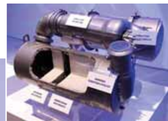
Komatsu displayed the technology behind its Tier 4 Final engines, including the selective catalytic reduction components (inset) that reduce emissions to near zero.
