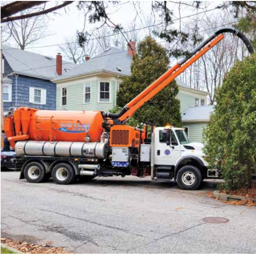
Portland, Maine's Department of Public Works also utilizes a Vactor 2100i combination sewer cleaner. "The combination machine is used to clean, vacuum and maintain 1.4 million feet of sewer pipe annually," said Utility Coordinator John Emerson.
