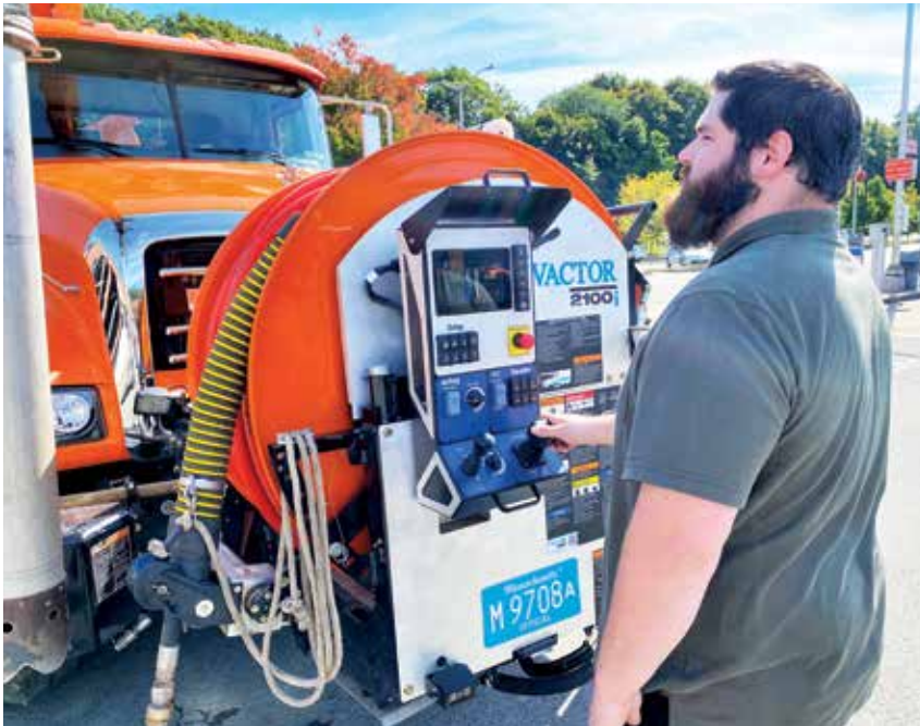
Fleet Supervisor Brian Zabchuk operates the RDB 1015 Rapid Deployment Boom on the Vactor 2100i combination sewer cleaner with the control panel on the front of the vehicle.
